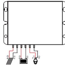
1. Follow the chart, connect the load (positive pole and negative pole) with the corresponding brown and blue cables firstly, then seal them with tape.
